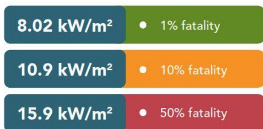
Figure 7 Heat flux and fatality levels, outdoor, for a 60s exposure
